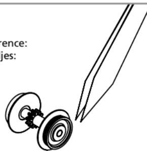
If used frequently, oil the wheelsets with a drop of non-resinous, acid-free sewing machine oil! In order to achieve the best possible running and traction properties, it is advisable to run the locomotive in forward 25 minutes and reverse 25 minutes without load. Clean rails are essential for good performance.
